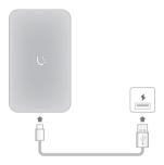
Plug USB-C end of cable into Prelude USB-C port. Plug USB-A end of cable into power adapter (not included).
